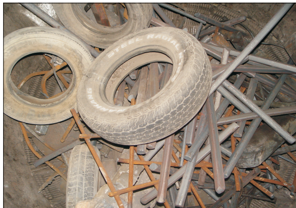
Fig. 4. Charging of scrap tires in scrap basket
