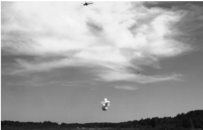
Fig. 8. Explosion of the water-capsule 16 meters over the ground – based on the registered film
