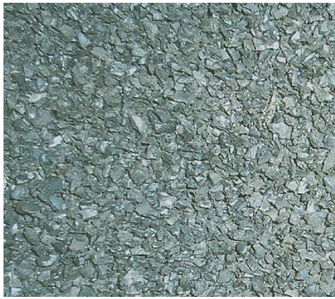
Fig. 1. Rubber granulate: volumetric density: 458 \text{ kg/m}^3 , grain size: 2 \times 4 \text{ mm} , grain shape: irregular flakes, fine-grained type
