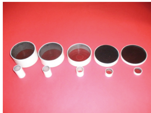
Fig. 4. A set of sleeves to examine sound absorbing properties for five layer thickness values (10, 20, 30, 40, 50 mm)
