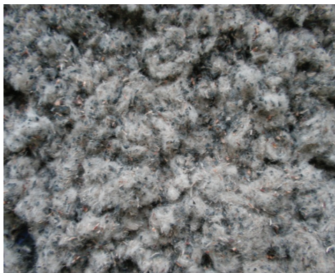
Fig. 2. Fabric-rubber granulate: volumetric density: 340 \text{ kg/m}^3 , rubber granulate contaminated with cotton fibre floccules, grain size: 2 \times 4 \text{ mm}
