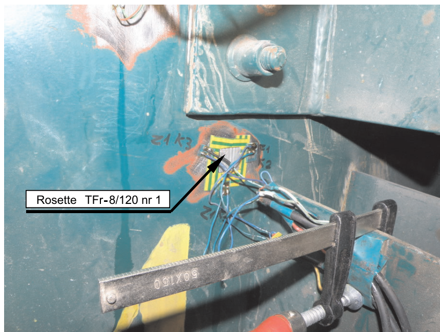
Fig. 11. Rosette 1 mounted in the bottom part of the separator's lower support
