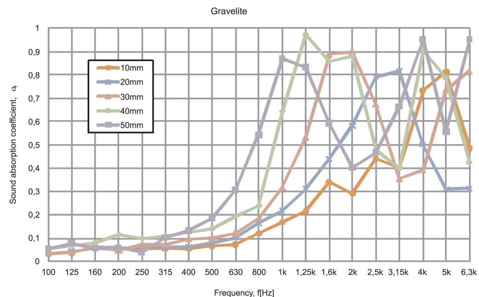
Fig. 5. Comparison of sound absorption characteristics of granular gravelite for various layer thicknesses
