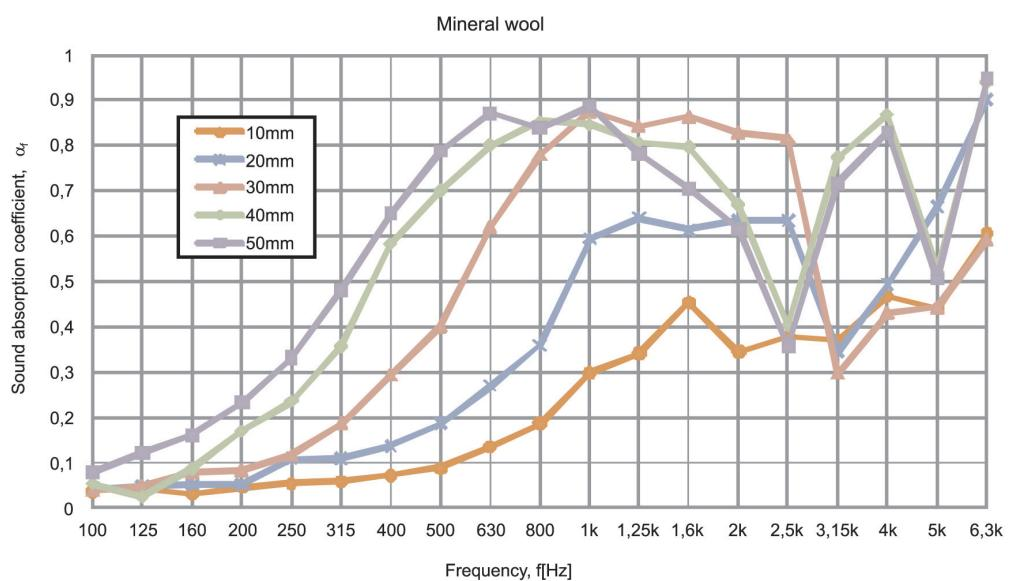
**Fig. 7.** Comparison of sound absorption characteristics of mineral wool granulate for various layer thicknesses
