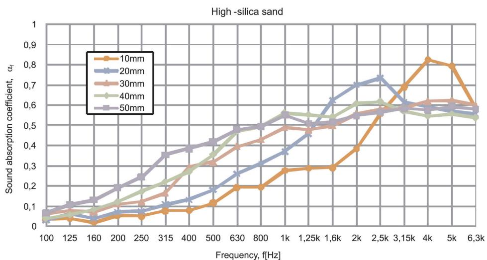
**Fig. 8.** Comparison of sound absorption characteristics of high-silica sand for various layer thicknesses
