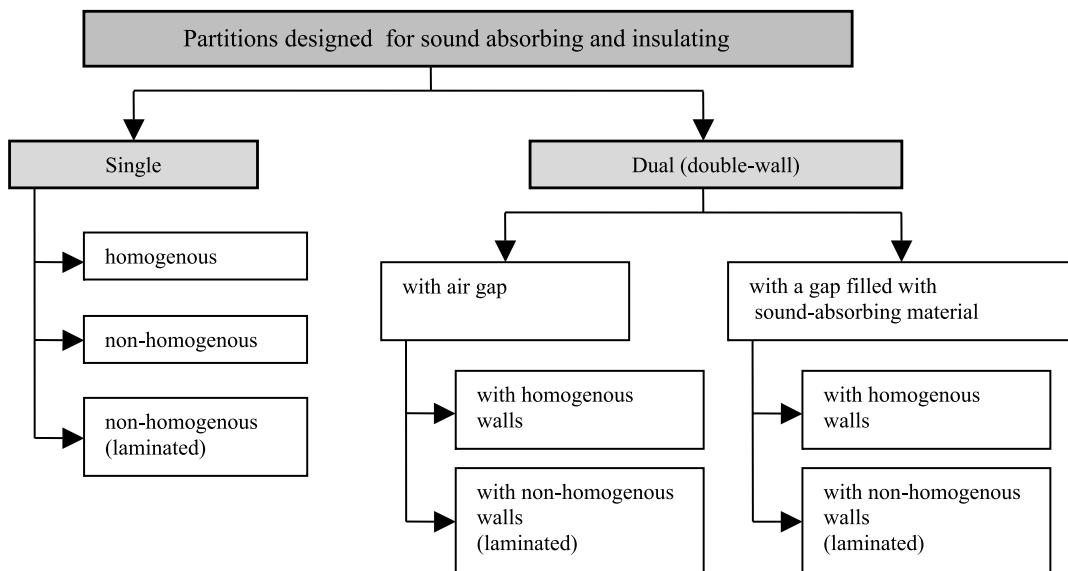
**Fig. 1.** Classification of sound insulating and sound-absorbing insulating partitions designed in solutions of classical and integrated enclosures
