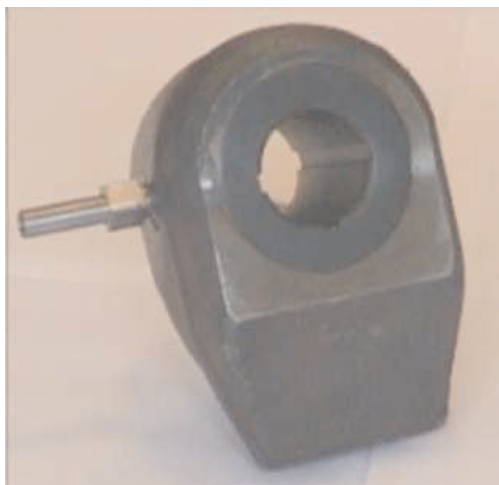
Fig. 8. View of modernized, lubricated holder for the tangential rotary tools of the RM 8 system used for tests (Bęben et al. 2001; Kotwica, 2003, 2005)
