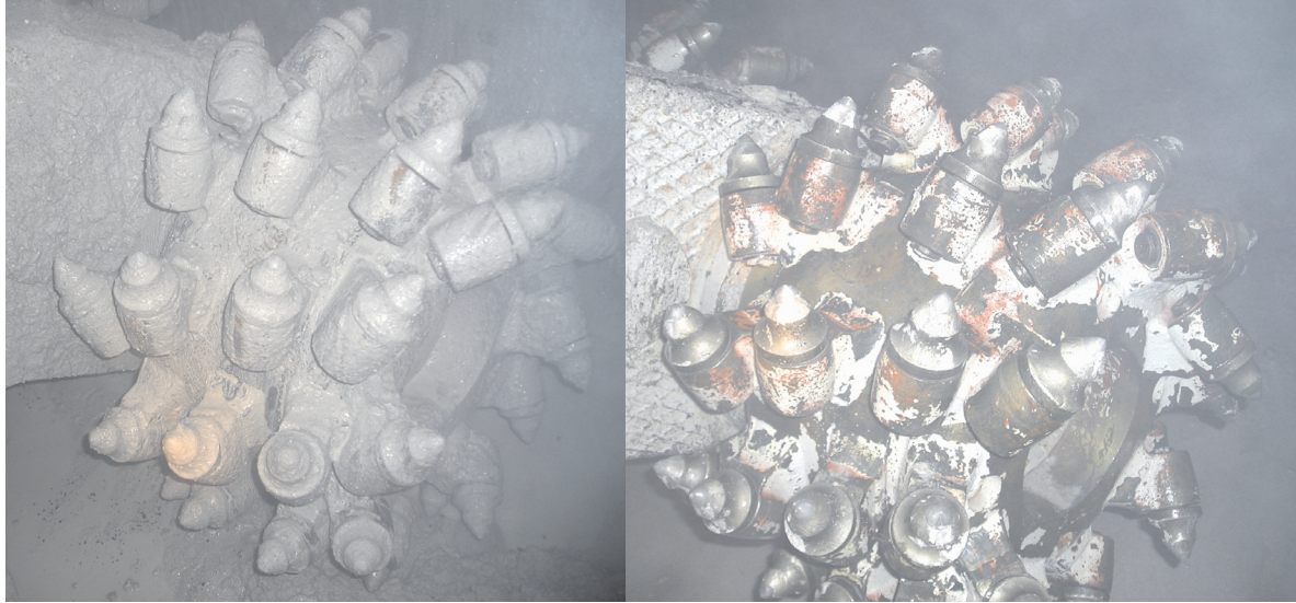
Fig. 18. View of the “dirty” cutting head of AM-50 roadheader with standard holders after mining (left) and the “clear” cutting head with lubricated holders after mining (right)
