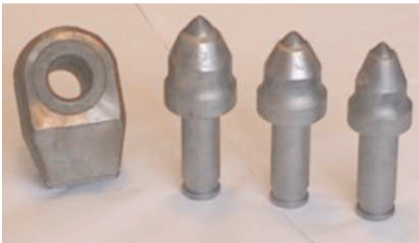
Fig. 5. View of RH8 tool-holder and tangential picks RM8 V5, RM8-520, Alpine (Kotwica 2003)
