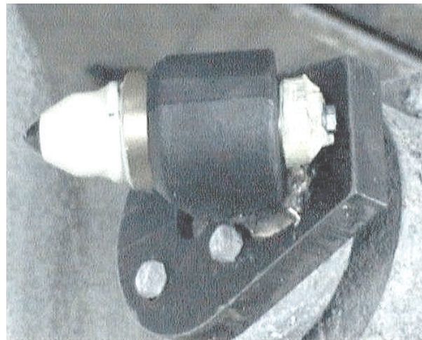
Fig. 9. View of bearing holder with the supportive bearing globule in the holder used for tests (Bęben et al. 2001; Kotwica 2005)
