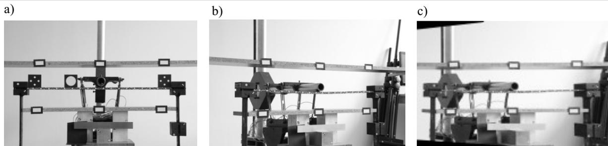
Fig. 3. The reference image (a) the image captured from a different point in space (b) the image rectified by the homography matrix (c)
