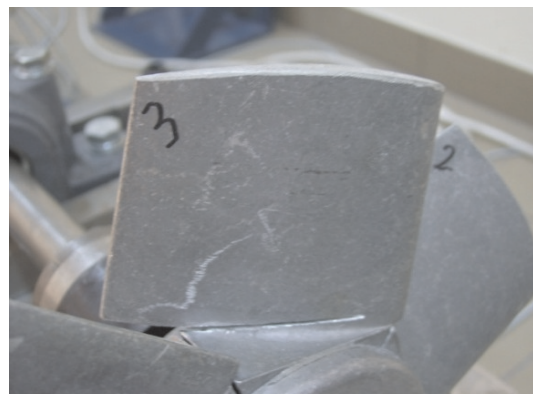
Fig. 12. Simulation of crack at blade no 3
