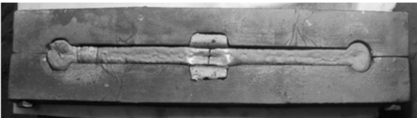
Fig. 23. Metal mould for researching hot tears
