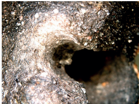
Fig. 3. Macroscopic picture of mould (accession no. 64/78) different sizes of sand grains visible, magnification 7x
