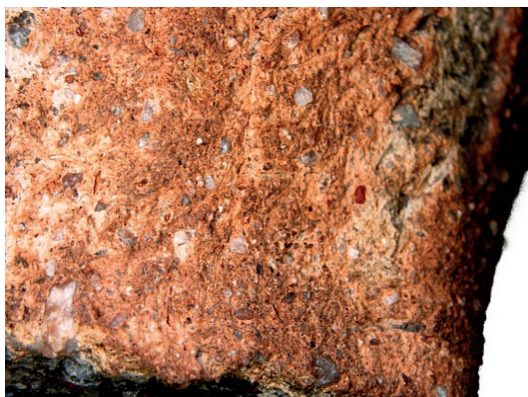
Fig. 4. Macroscopic picture of mould (accession no 64/78) different sizes of sand grains visible, magnification 50×
