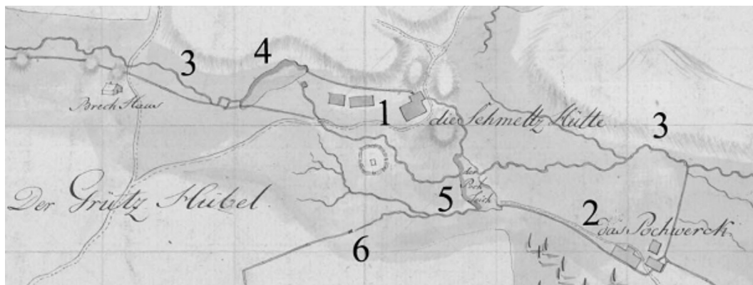
Fig. 6. A fragment of a map of Miedzianka from 1784 (tracing from 1784) with the area of Jagwitz smelter marked (OBB II 1072). 1 – smelter buildings, 2 – ore-stamp mill buildings, 3 – the course of Miedzianka brook, 4 – pond for smelting, 5 – pond for ore-stamp mill, 6 – an inlet of Neu Glück. Collection of National Archives in Katowice
