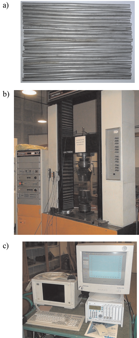
Fig. 1. Tensile specimens (a) and Instron 1196 testing machine (b) with measuring apparatus (c)
