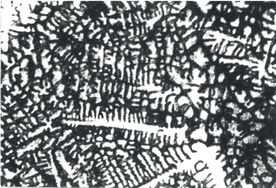
Fig. 10. Microstructure of polymetallic alloy from Series of Tests No. 4 (mag. 250×)
