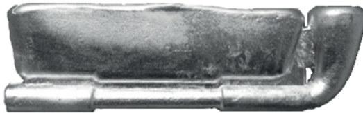
Fig. 2. Round sample for tensile tests with gating system and riser
