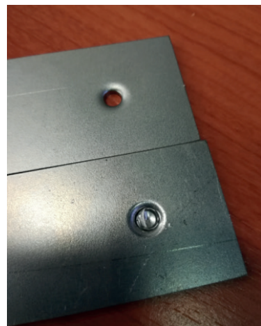
Fig. 15. After test – full shear mode
