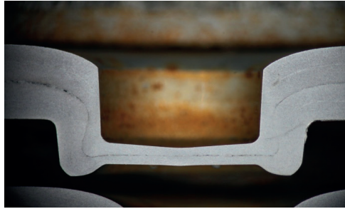
Fig. 8. High forming force; tB = 0.46 \text{ mm}
