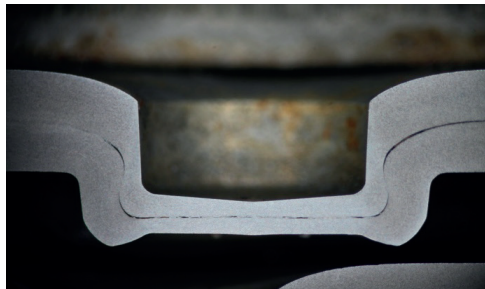
Fig. 10. Small undercut; tB = 0.65 \text{ mm}
