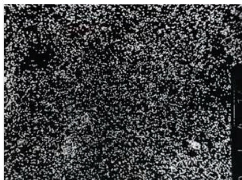
Fig. 12. The surface distribution of manganese in silicon bronze \text{CuSi}_3\text{Zn}_3\text{MnFe} of ingots metallurgical (magn. 1000 \times )
