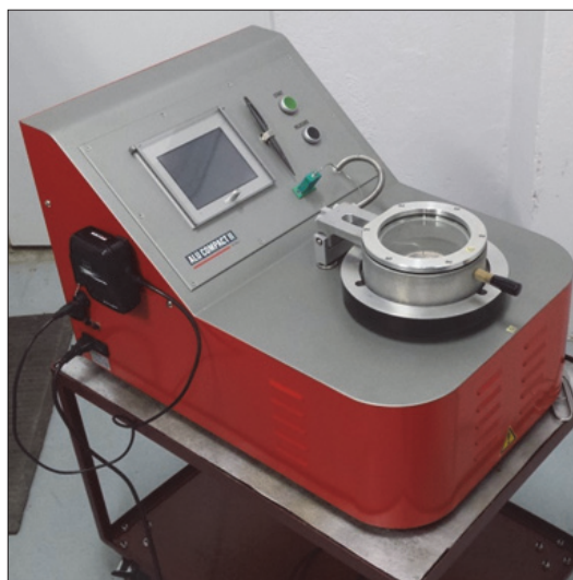
Fig. 4. Devices for assessing the gassing degree: a) ALU COMPACT II; b) GAS-METER
