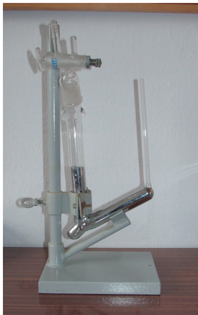
Fig. 2. Test stand for determination of diffusible hydrogen content by mercury method
