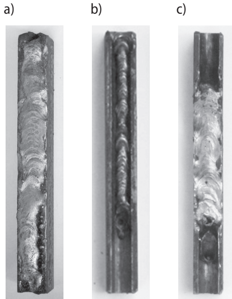
Fig. 3. Samples for diffusible hydrogen content determination: a) sample with four weld beads (ER + ER + ER + ER); b) sample with one weld bead (EC); c) sample with four weld beads (EC + EB + EB + EB)
