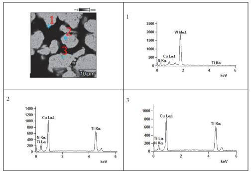
Fig. 2. EDS analysis after 20 h of mechanical alloying, magnification 3000×
