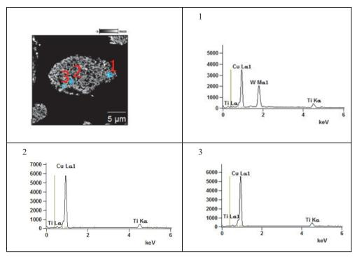
Fig. 4. EDS analysis after 30 h of mechanical alloying, magnification 5000imes
