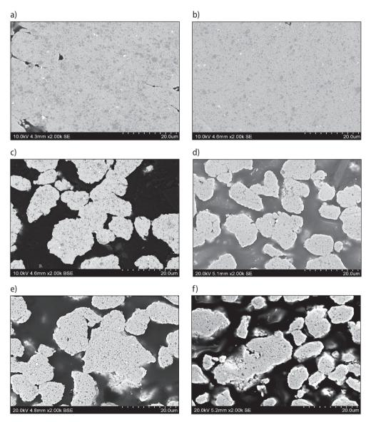
*Fig. 1. SEM microstructures of Cu-10 wt.% TiN composite powders: a) 5 h mechanical alloying, magnification 2000×; b) 10 h mechanical alloying, magnification 2000×; c) 15 h mechanical alloying, magnification 2000×; d) 20 h mechanical alloying, magnification 2000×; e) 25 h mechanical alloying, magnification 2000×; f) 30 h mechanical alloying, magnification 2000×*
