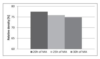
Fig. 5. Influence of milling time on relative density of Cu-10 wt.% TiN
