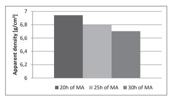
Fig. 6. Influence of milling time on apparent density of Cu-10 wt.% TiN
