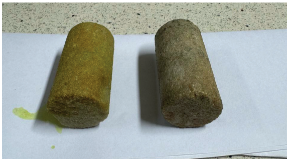
Fig. 2. Difference in color between the core sample treated with hydrochloric acid (left) and the untreated core sample (right)
