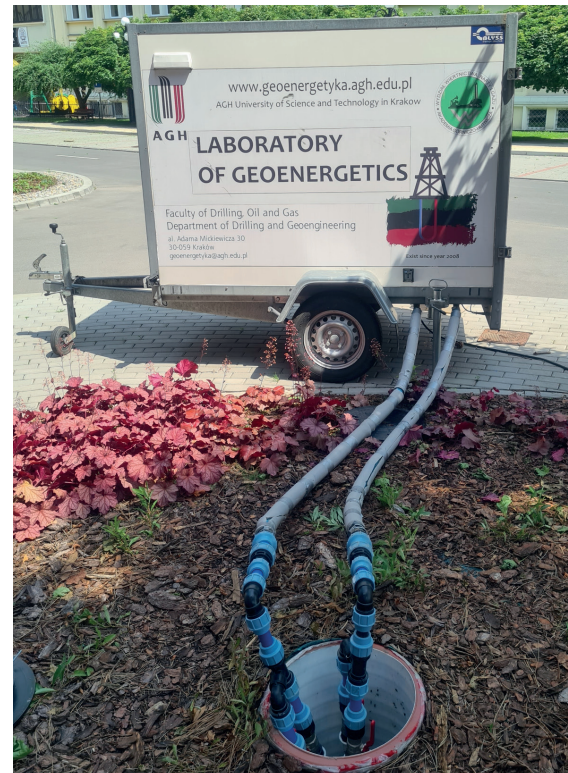
Fig. 1. TRT Equipment (photo Geoenergetics Lab team)
