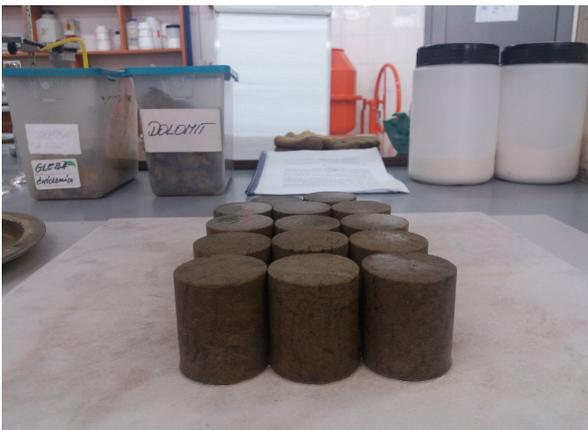
Fig. 2. Prepared core samples
