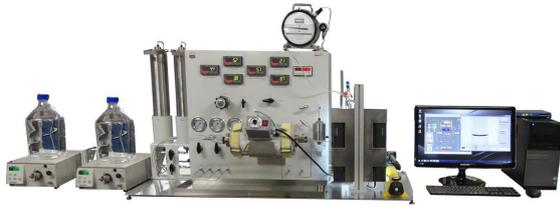
Fig. 1. Bench-top relative permeability system
