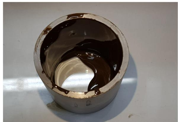
**Fig. 5.** Bushing with layer of oil mud inside
