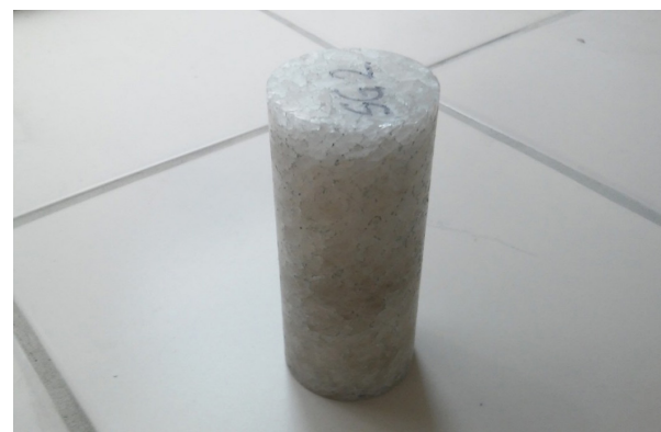
Fig. 6. Salt sample SG2. The picture shows a disorderly, medium-crystalline salt structure
