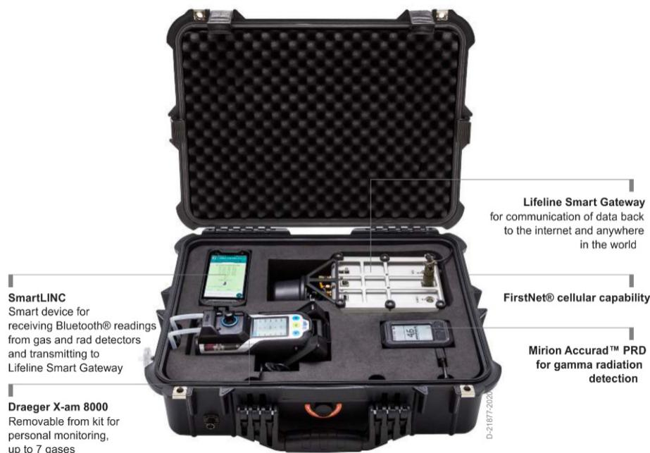
Fig. 9. Dräger X-site Live set contents [40 – modified]
