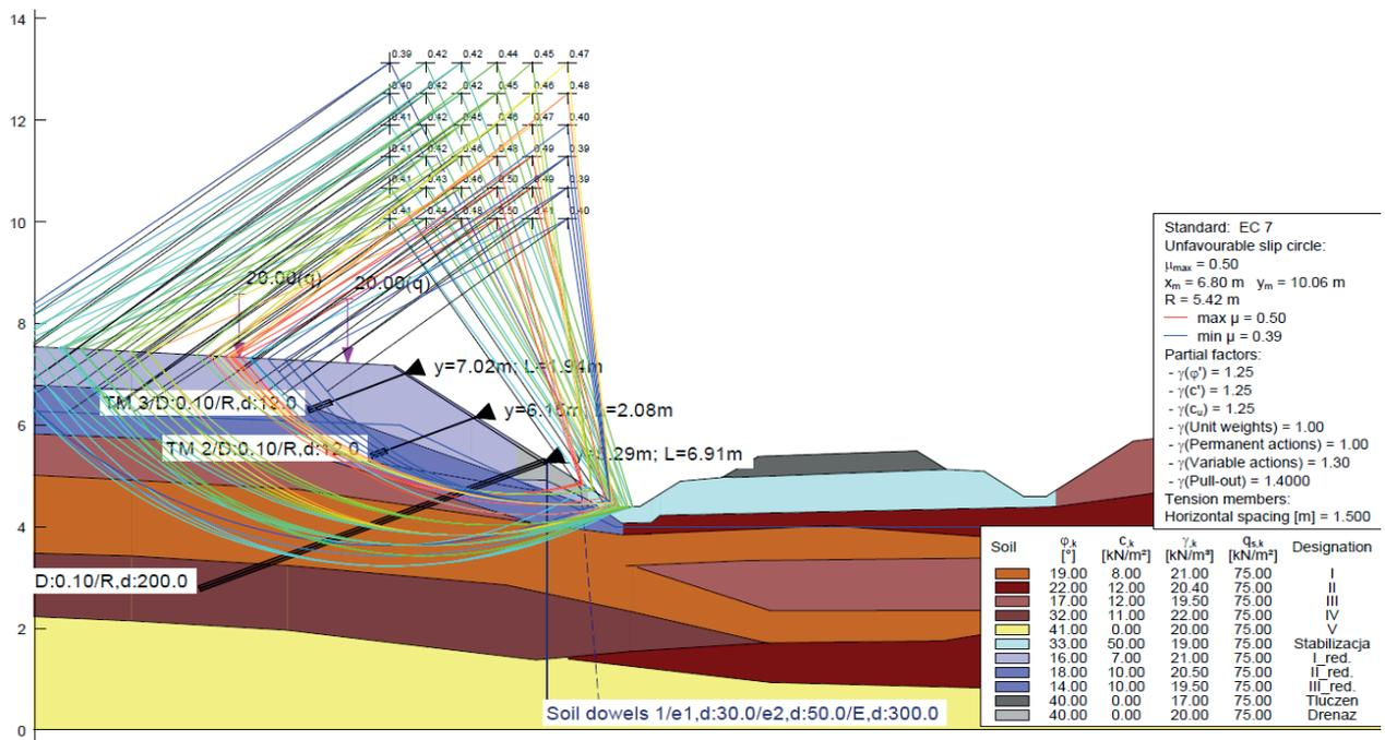
Fig. 10. View of design cross-section with calculations for selected point 33+400 (Geotechnical project BAARS, 2020)
