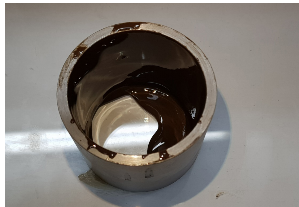
Fig. 5. Bushing with layer of oil mud inside
