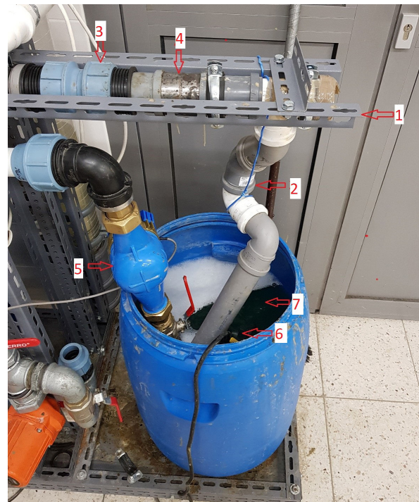
Fig. 4. Washing device used for the laboratory research: 1 – a metal frame; 2 – hydraulic system consisting of PCV pipes; 3 – pipes with spacer nuts; 4 – steel bushing during washing; 5 – electrical device measuring the flow rate; 6 – submersible pump Viper 2850 WQD-10-8-0.55; 7 – pre-flush in plastic barrel
