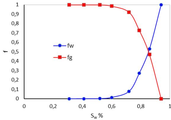
Fig. 4. The fractional flow curves for the relative permeability data of Figure 2
