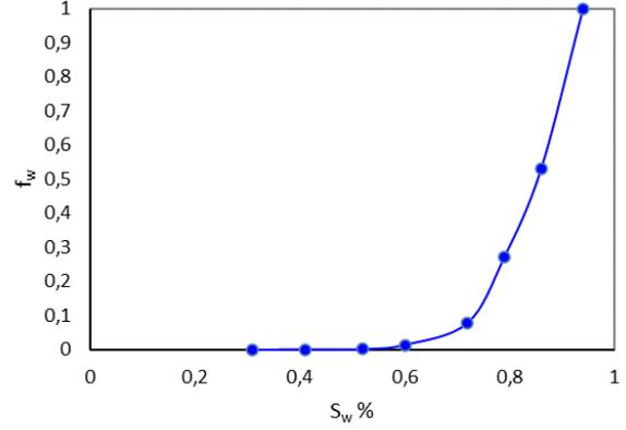
Fig. 3. Water fractional flow curve for the relative permeability data of Figure 2
