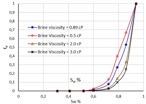
Fig. 6. The effect of brine viscosity on  $f_w$  behavior
