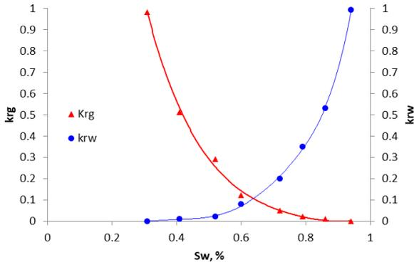
Fig. 2. Gas-water relative permeability curves
