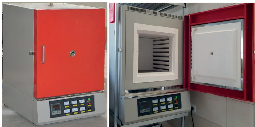
Fig. 2. KJ-M1200-64L-IC muffle furnace used for heat treatment of the welded joint samples
