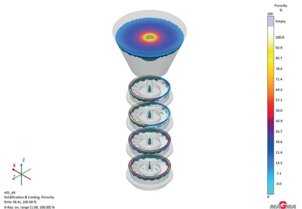
Fig. 17. Porosity distribution for the redesigned configuration (Design 4)
