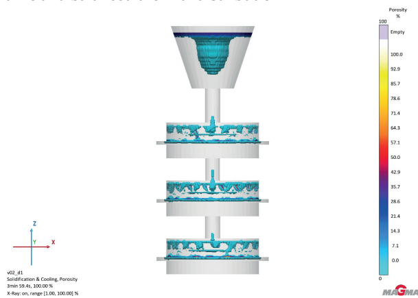
Fig. 20. Porosity distribution for the initial design (Design 1)
