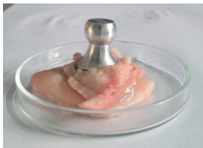
Fig. 6. A sample of bonded porcine tissues prepared for pull-off adhesion testing
