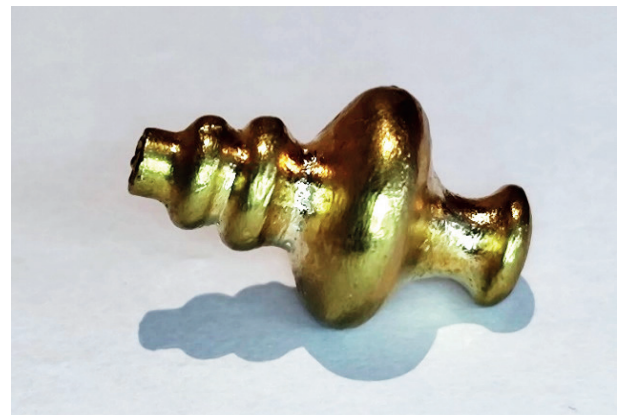
Fig. 9. Casting obtained using the investment casting method
