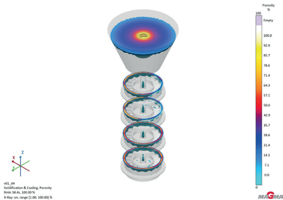
Fig. 17. Porosity distribution for the redesigned configuration (Design 4)
