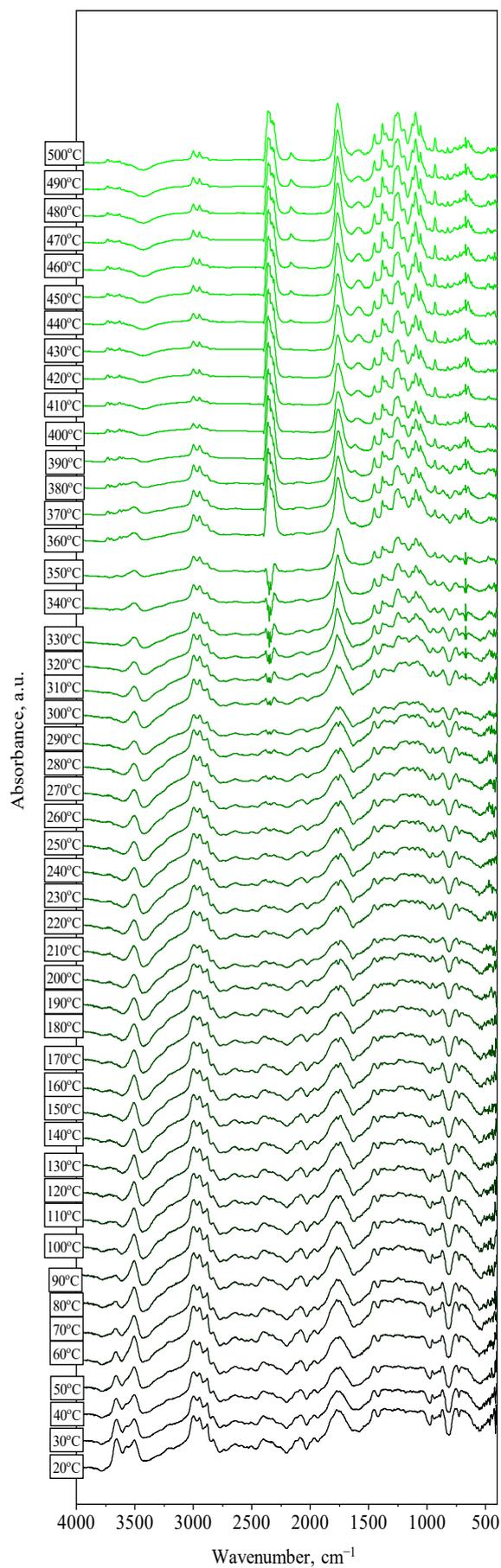
Fig. 7. DRIFT spectra of PLA7
