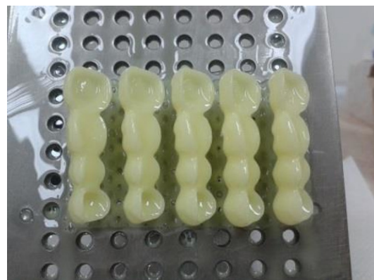
Fig. 1. 3D printed cast patterns of dental bridges [3]
