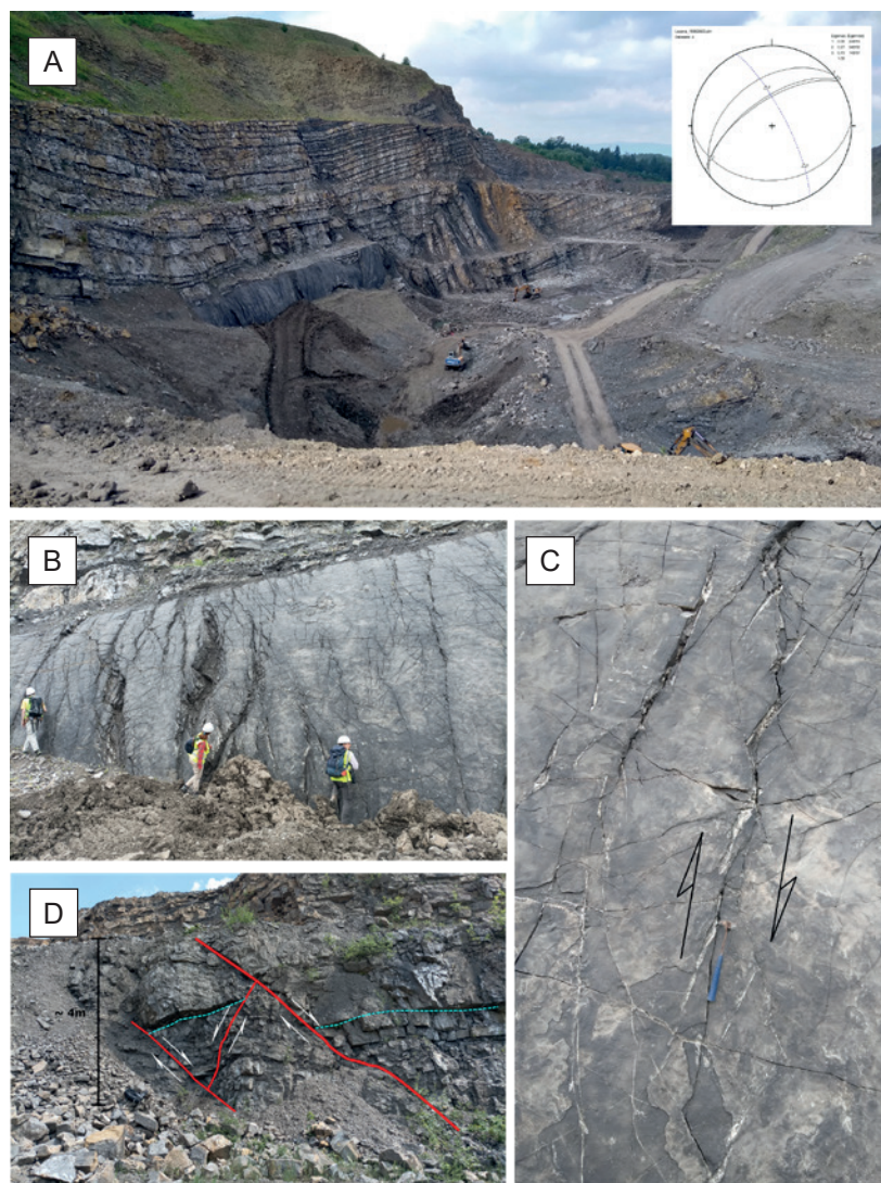
Fig. 20. Selected tectonic structures in the Leszna Górna quarry: A – a fold structure proving NNW shortening; B – hinge zone of the fold in picture A, with well-visible dextral shear zones (C) (hammer for a scale); D – conjugate set of normal faults formed as a result of fold axis-parallel extension.
