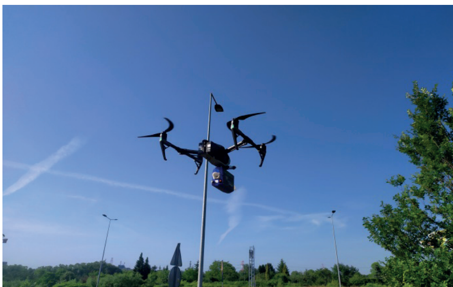
Fig. 1. UAV platform for measuring traffic-related pollution
