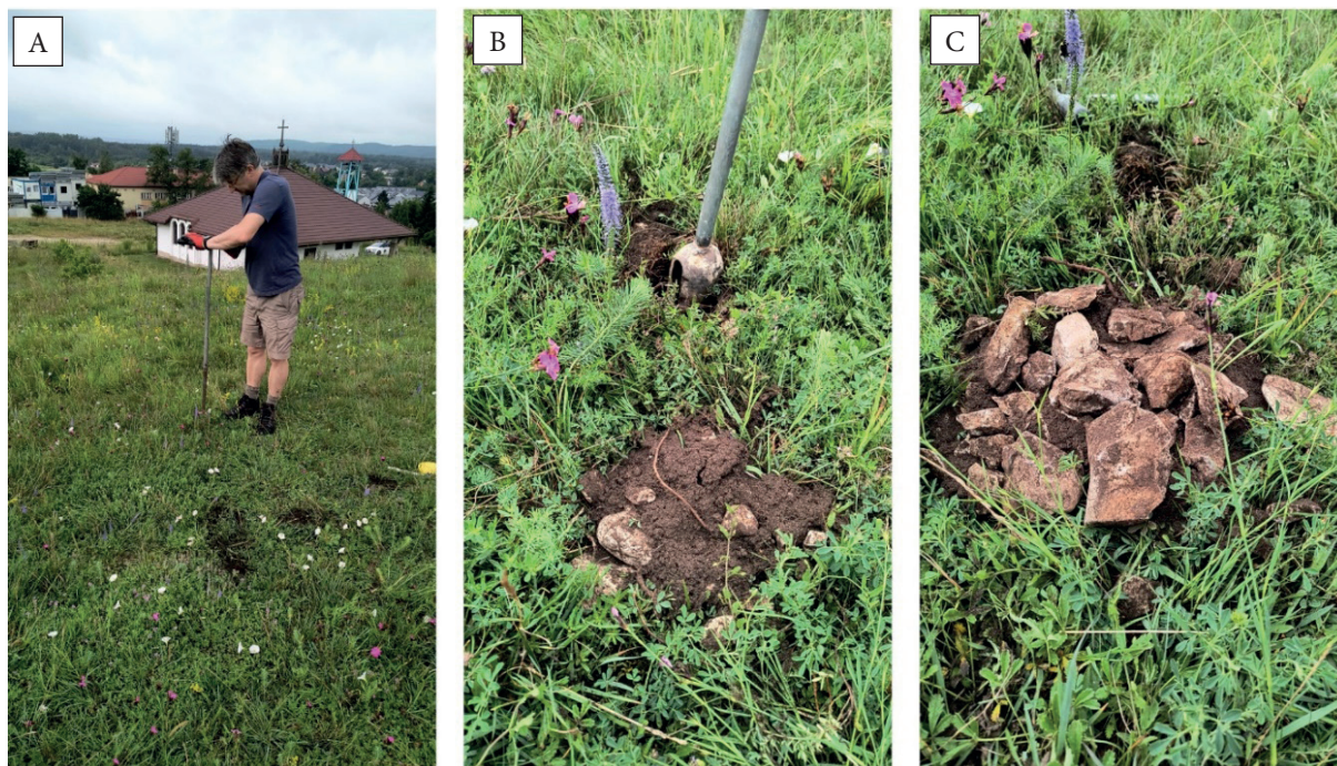
Fig. 11. Verification drilling in the investigation site, named “The cavern under the chapel” (A); geological material taken from depths 0–0.5 m (B) and 0.5–1.0 m (C)
