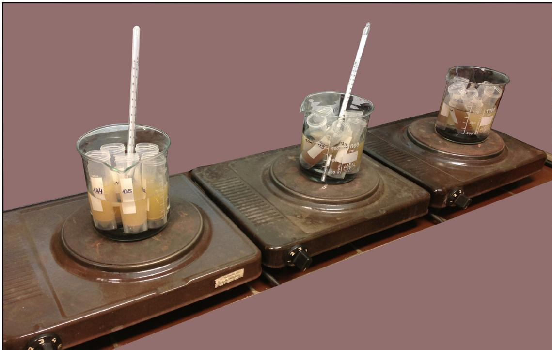
Fig. S3. Test tubes with a mixture of ash and HCl acid in a water bath (photo by D. Tsvirko, 2022)
