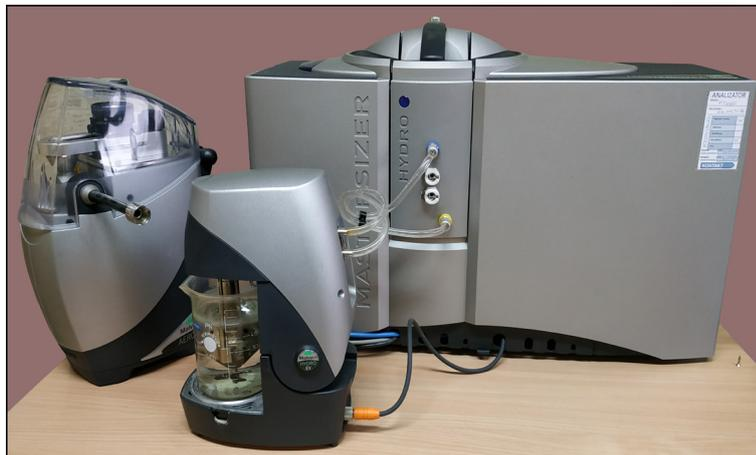
Fig. S10. Malvern Panalytical Mastersizer 3000 for laser textural (particle size distribution) analysis (photo by D. Tsvirko, 2022)
