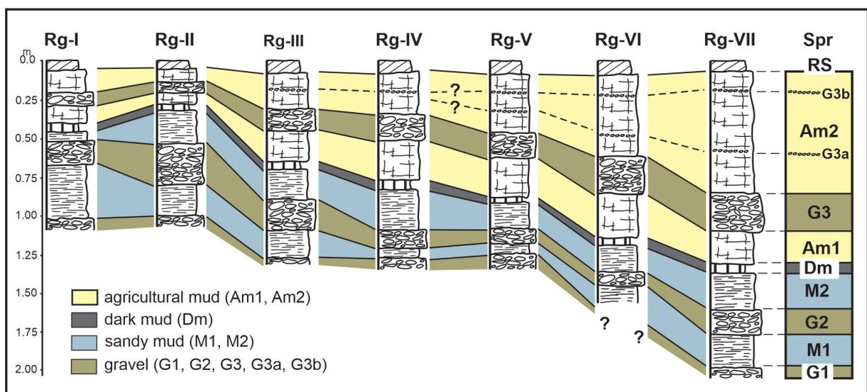
**Fig. 5.** Longitudinal section of the low terrace of the Rogoźnik Stream valley (see also Figs. 2, 3 and 4): Spr – synthetic lithological profile, M1, M2 – sandy-mud horizons (described in text), G1–G3 – gravel horizons (described in text), G3a, G3b – gravel inserts (described in text), Am1, Am2 – silty-mud horizons (agricultural mud) (described in text), Dm – dark mud horizon (described in text), RS – recent soil, Rg-I – Rg-VII – profiles of fluvial deposits
