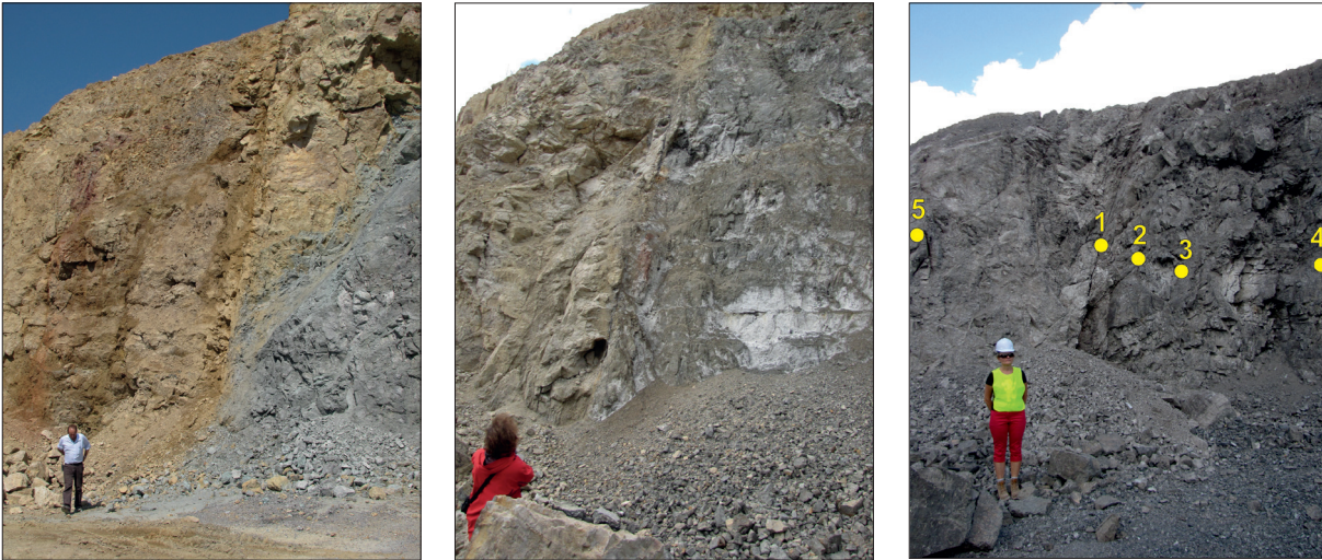
Fig. 3. NNE-SSW fault in the Budy Quarry at III, IV and V exploitation level: 1-5 – sample location (see Table 1)
