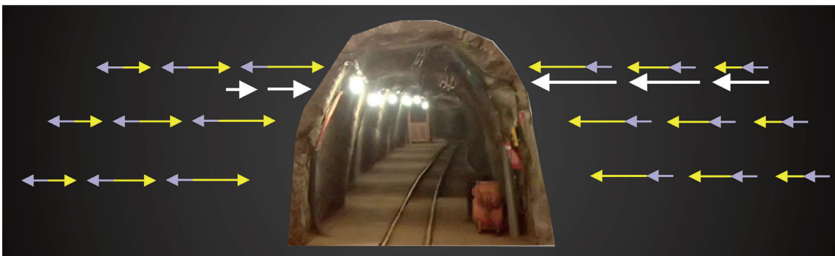
Fig. 14. The distribution of modeled displacement vectors determined on the basis of the measurements: the white arrows are displacement vectors whose rates were determined by the extensometric measurements, the yellow arrows are displacement vectors resulting from the process of convergence, the cyan arrows are displacement vectors resulting from the tectonic push
