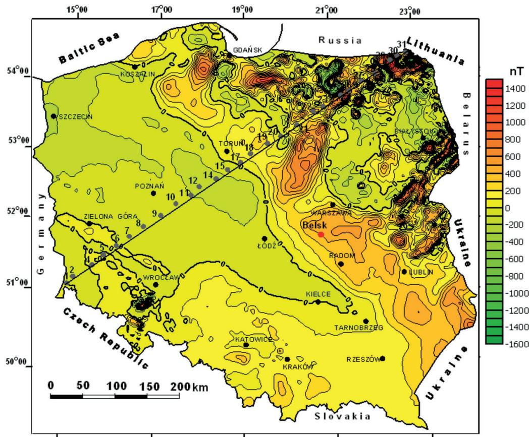
Fig. 2. Location of the measurement sites (secular points) along the Zgorzelec-Wizajny (Z-W) profile on the background of the magnetic map ( $\Delta Z$ ) of Poland, contour interval 100 nT, grid  $5 \times 5$  km (Bojdys & Grabowska 2007). Data source: Karaczun et al. (1978)
