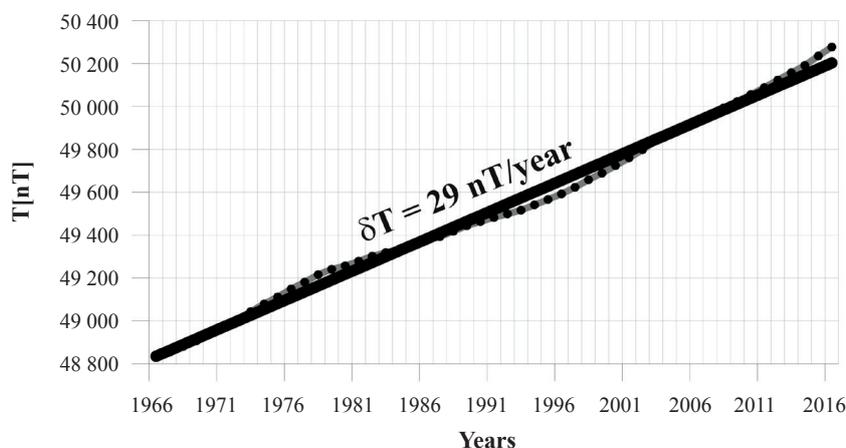
**Fig. 6.** Variations of the geomagnetic field intensity ( $T$ ) through the years 1966–2016 at the Central Geophysical Observatory in Belsk with the mean variation ( $\delta T$ ) [nT/year]
