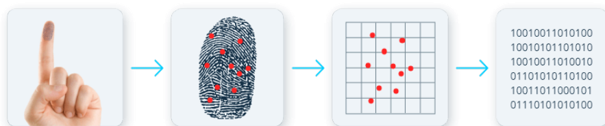
Figure 3. The process of extracting binary data from a fingerprint [9]
