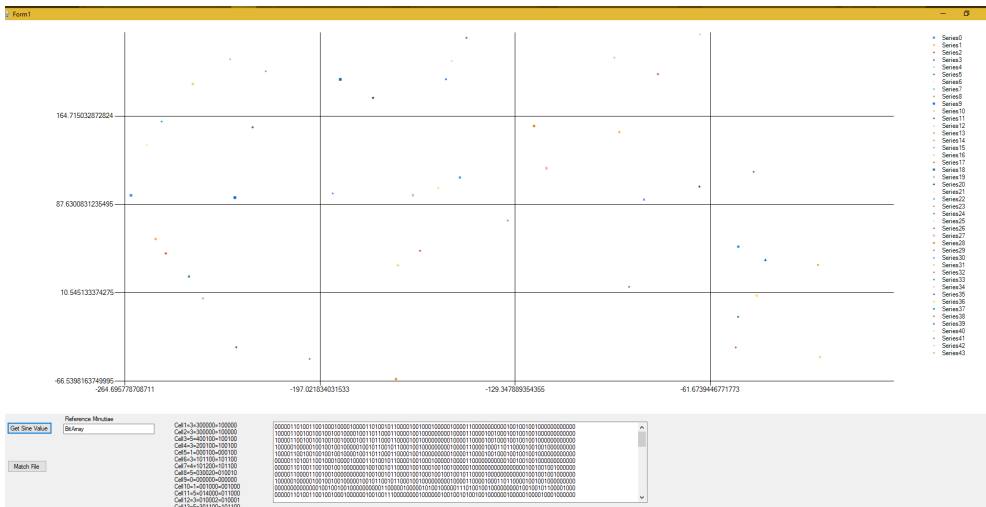
Figure 3. Screenshot from implemented solution where new coordinate system is tessellated into equal-sized grids
