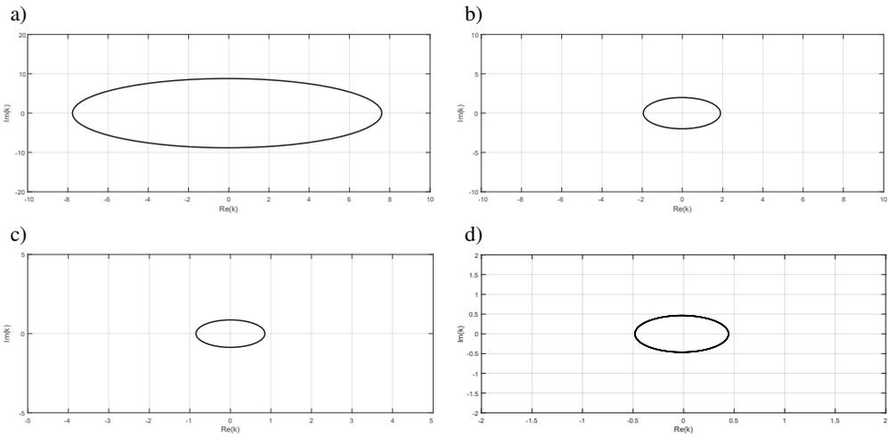
**Fig. 5.** D-decomposition regions for discrete-time subsystem: a) discrete-time for  $v_1$ ; b) discrete-time for  $v_2$ ; c) discrete-time for  $v_3$ ; d) discrete-time for  $v_4$
